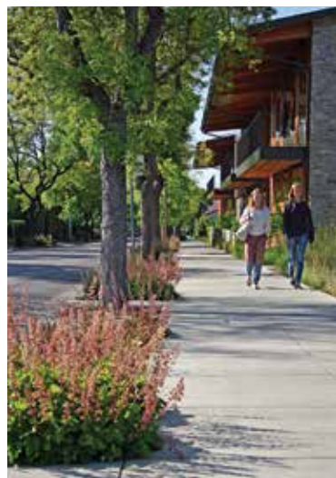
RIGHT Rain gardens on a side street are planted with Heuchera , Juncus , and other natives to capture and filter stormwater.
